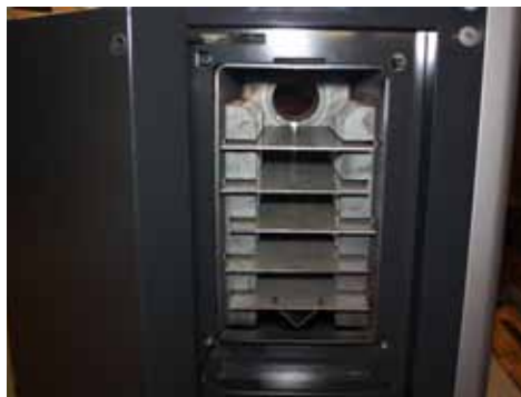
Open the convection cleanout hatch.
