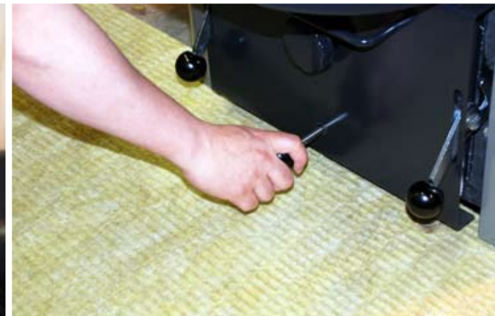
Ash compression lengthens the interval between emptying the ash. The ash tightens when the adjuster is moved back and forth.
