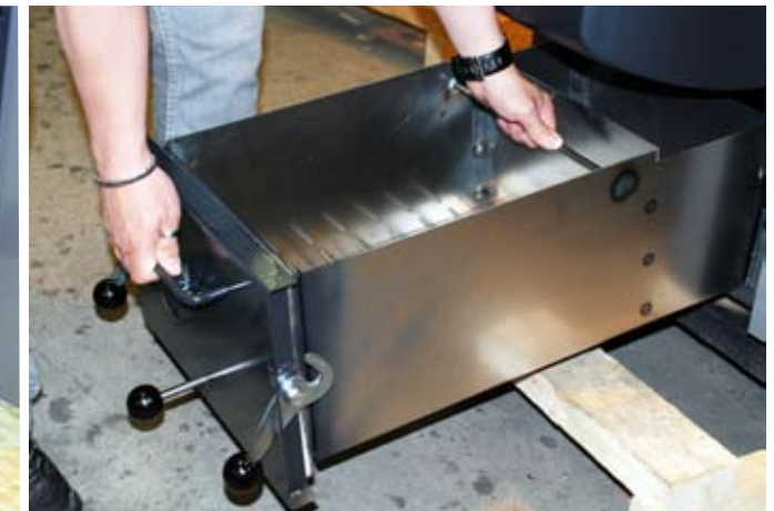
Emptying the ash. Pull out the ash box. Empty the ash into a decked fire-proof container outdoors. Because of the fire risk, the container must not include anything but ash.
